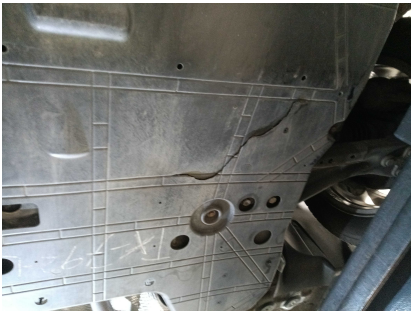
3. BODY - FRONT SECTION: Damaged engine cover
