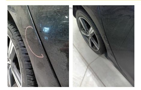
2. SIDE: Left and right side - visual damage / scratches
