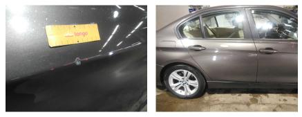
3. SIDE: Left and right side - visual damage / scratches
