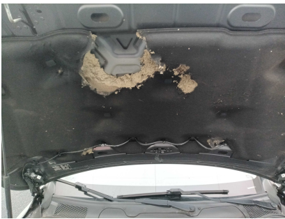
5. FRONT: Hood sound insulation for condition
