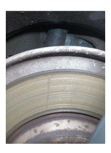
**2. BRAKES:** Front brake disc (both)
