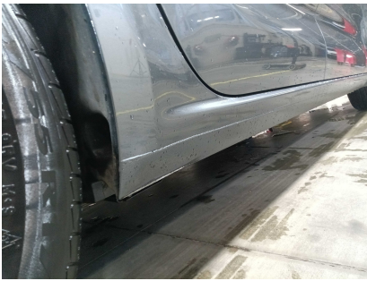
3. SIDE: Left and right side - visual damage / scratches
