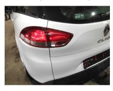
**3. LIGHTS:** Rear lights (brake, fog, indicator) - basic functioning, damage, color
