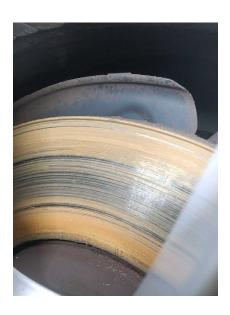
2. BRAKES: Rear brake disc (both)
