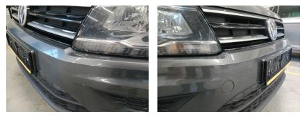
4. SIDE: Left and right side - visual damage / scratches
